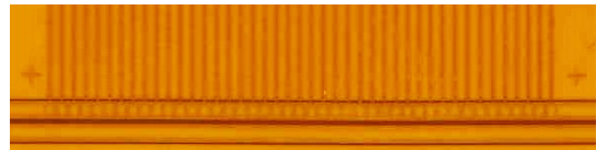
MWM-Array for high resolution surface crack imaging of SCC colonies
